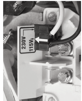
Figure 4B Voltage Change Plug Set for 115 Volts
