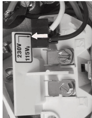
Figure 4A -Voltage Change Plug Set for 230 Volts
