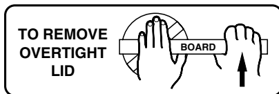
Figure 6 – Use a pry bar or board as shown to remove tight lid. Do not use a pry bar to tighten lid.
