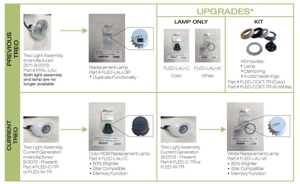
\*Upgrade kits are available to bring previous generation Treo light assemblies up to the current generation. If you have the previous generation lamps (FLED-LAU-DIP), and desire to upgrade to the current generation, you must change **ALL** the lamps to the current generation (FLED-LAU-C/W) for proper synching and consistent brightness.
