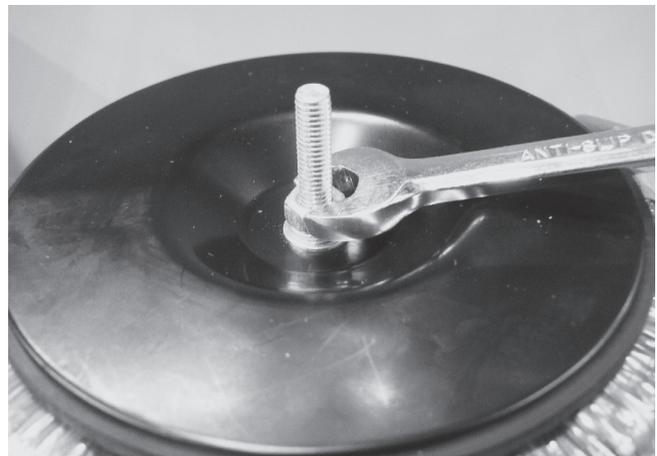
**Step 2** – Place heat dispersion disk over the transformer with the shiny metallic side face up. Place flat washer in place over the locating screw, tighten the transformer nut using an 8mm spanner.
