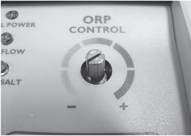
**Step 3** – When PCB is in place the ORP control holder will be visible poking through the front panelling. Reconnect ORP control knob to its holder ensuring it is able to be adjusted to both minimum & maximum settings.
