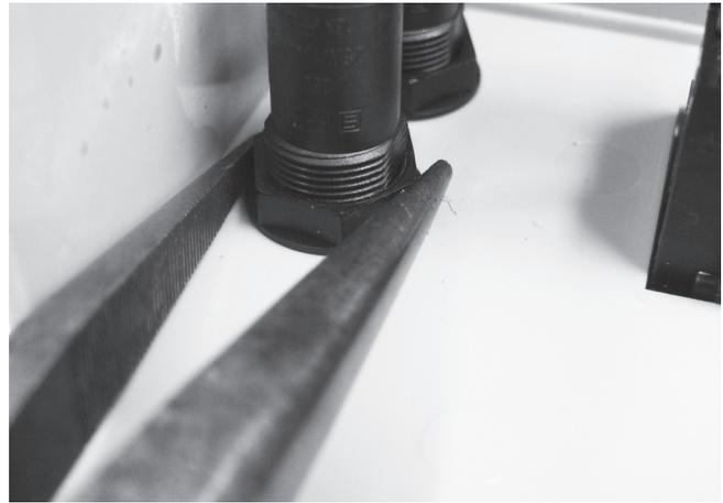
**Step 2** – Using a pair of long nose pliers undo the nut holding the fuse housing in place.
