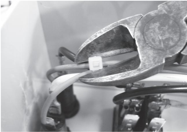
**Step 1** – Remove all applicable cable ties with a pair of side cutters. Take special care not to cut or damage the wiring.
