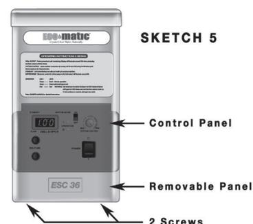
When replacing the front panel, be sure that all internal wiring is clear of the side and bottom panels, to allow proper seating of the front panel. Insert sides of front panel into the slots at each side, slide the front panel UP so its top edge slides under the top panel. When the front panel is in place, re-tighten screw and replace circular cover plate.
