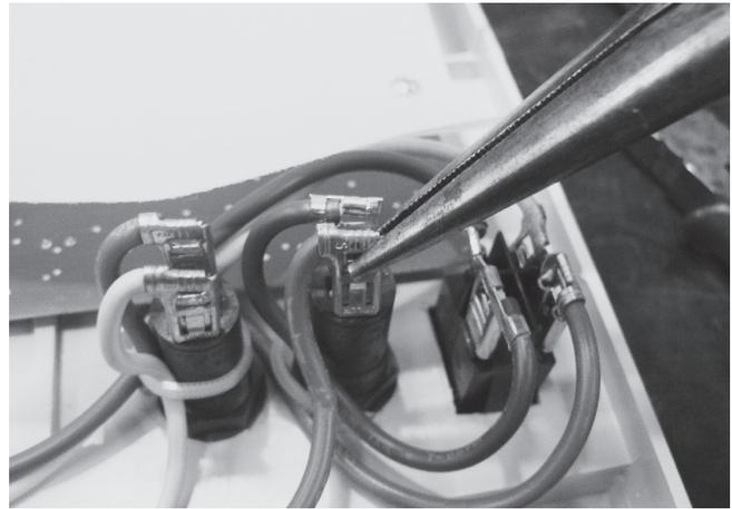
**Step 2** – Remove the terminal clips from the fuse housing.
