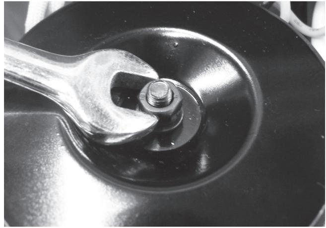
**Step 6** – Remove the nut on the top of the transformer with an 8mm spanner then lift off the black heat dispersion disk which when removed allows for the transformer to be lifted out of the chlorinator. When removing heat dispersion disk also remove both the spring & flat washers.
