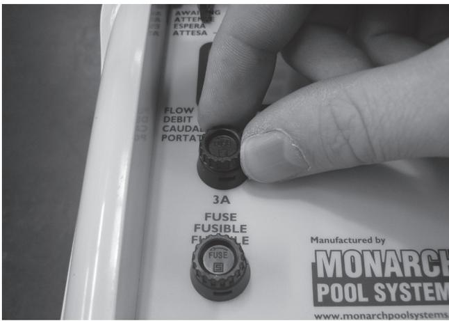
**Step 1** – Replace the fuse housing.
