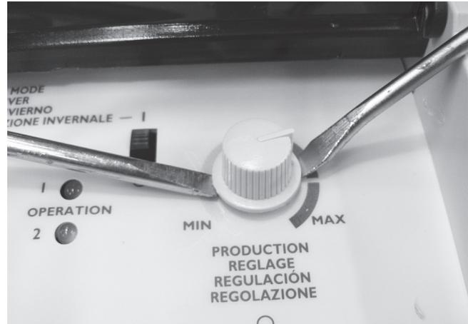
**Step 2** – Remove the sanitiser output knob which will allow you to move the PCB to the side. May need to use two flat blade screwdrivers to lever the knob off if it is fastened too tight to remove by hand. If using screwdrivers be careful not to damage the control panel.
