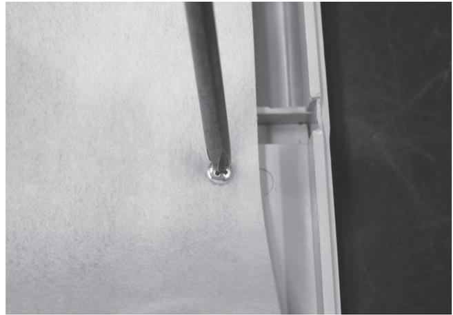
**Step 2** – Remove the screws holding the protective cover on the PCB with a Phillips head screwdriver (one point).
