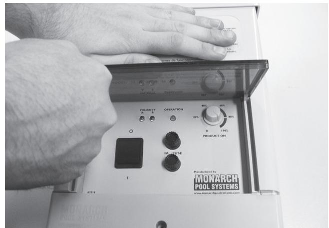
**Step 1** – First attach the door to the right hand lug then with the door completely upright push down on the left side to clip the door in place over the right lug. Check door opens & closes completely to check correct installation.
