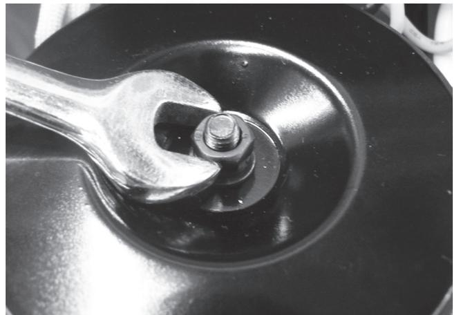
**Step 2** – Place heat dispersion disk over the transformer with the shiny metallic side face up. Place flat washer in place over the locating screw with spring washer on top, tighten the transformer nut using an 8mm spanner.
