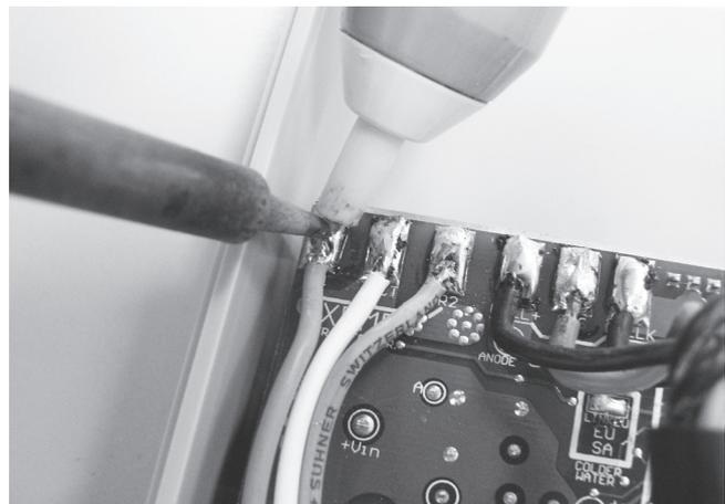
**Step 4** – With a soldering iron & solder sucker or solder wick remove the 3 transformer wires. The transformer wires are the orange, white & pink wires on the top left corner of the PCB. When the metal has cooled remove the transformer wires.
