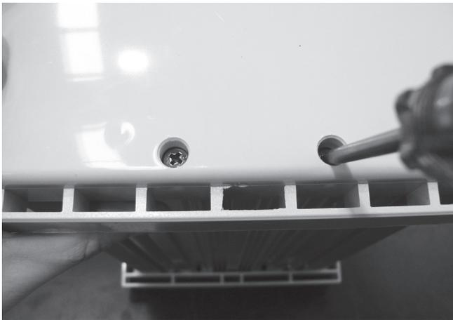
**Step 1** – Replace the screws holding down the top panel using a Phillips head screwdriver (two point).
