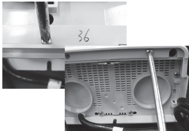
**Step 2** – Push the bottom of the front panel into place; panel is correctly placed when the screw connecting the two chlorinator halves can be placed through its connection & tightened. Reconnect front panel screws with a Phillips head screwdriver (two point).
