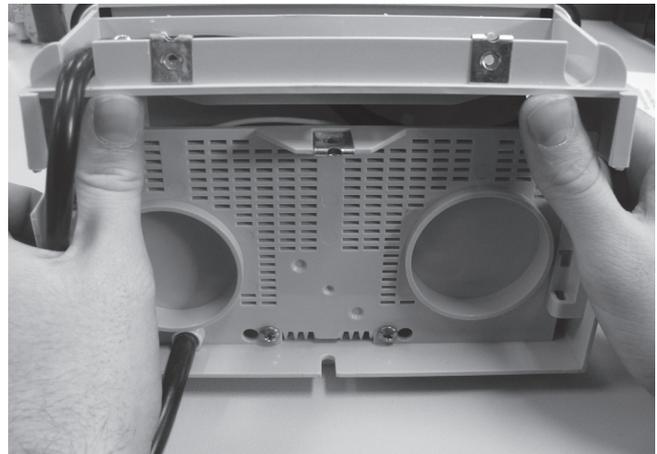
**Step 2** – Using both hands lift the front panel up & slide it out from the top panel, keep sliding until the top of the chlorinator comes free & the housing is able to be flipped open.
