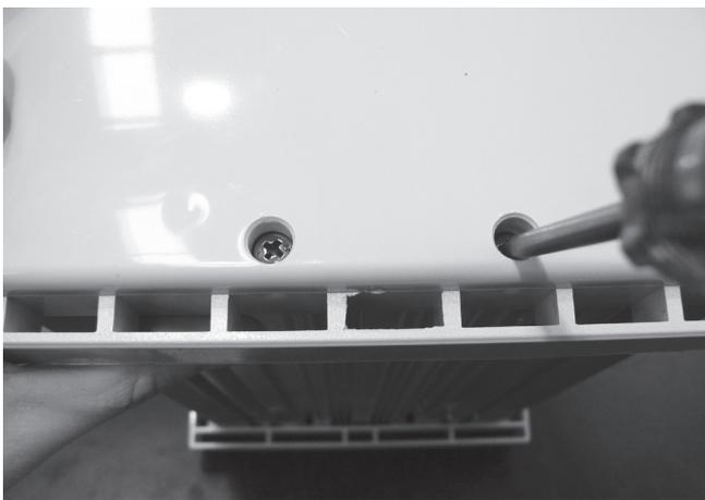
**Step 1** – Replace the screws holding down the top panel using a Phillips head screwdriver (one point) & press tabs back into place, (Part number M1500GRY).
