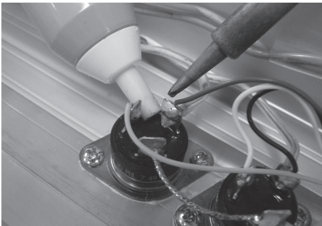
**Step 3** – Using a soldering iron & a solder sucker remove the wires connecting the transformer to the Triacs. Mark the wires to allow for easier reconnection.
