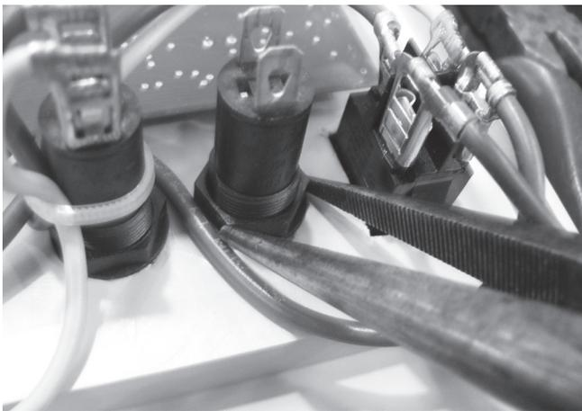
**Step 3** – Using a pair of long nose pliers undo the nut holding the fuse housing in place.
