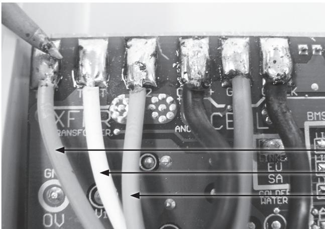
**Step 3** – After feeding the transformer wires through the clear tubing use a soldering iron with unleaded solder to attach the wires to the PCB. The order for connecting the wires from the left of the PCB is 1) orange, 2) white, 3) pink.
