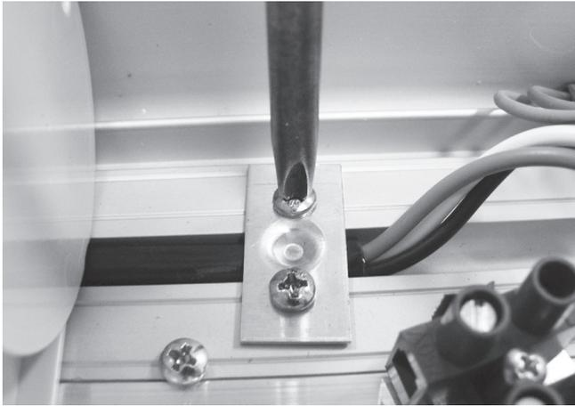
**Step 1** – Feed the power cord through the bottom panel & place power cord lead in correct position on the backing plate. Replace the holding plate using a Phillips head screwdriver (two point).
