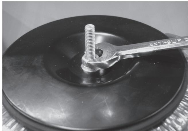
**Step 2** – Place heat dispersion disk over the transformer with the shiny metallic side face up. Place flat washer with the spring washer on top of it in place over the locating screw, tighten the transformer nut using an 8mm spanner.
