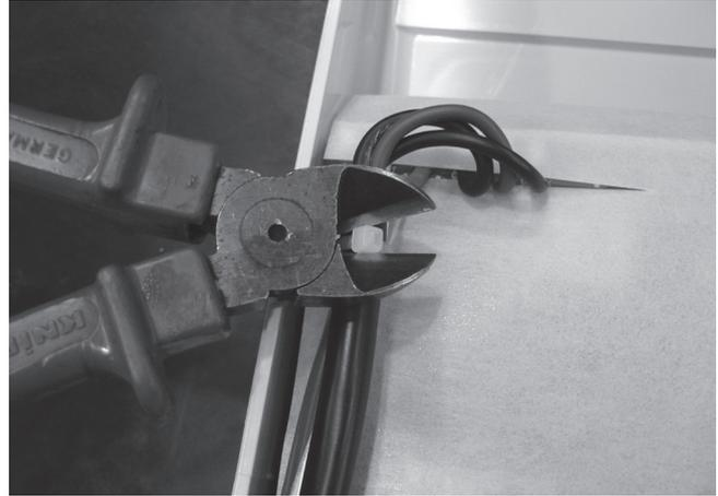
**Step 2** – Remove the appropriate cable ties with side cutters. Take special care not to cut or damage the wiring
