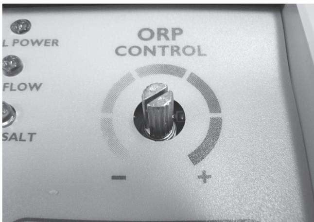
**Step 4** – When PCB is in place the ORP control holder will be visible poking through the front panelling. Reconnect ORP control knob to its holder ensuring it is able to be adjusted to both minimum & maximum settings.
