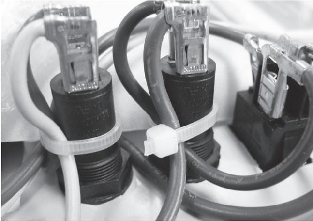
**Step 4** – Place cable ties into position holding the fuse wires in place.
