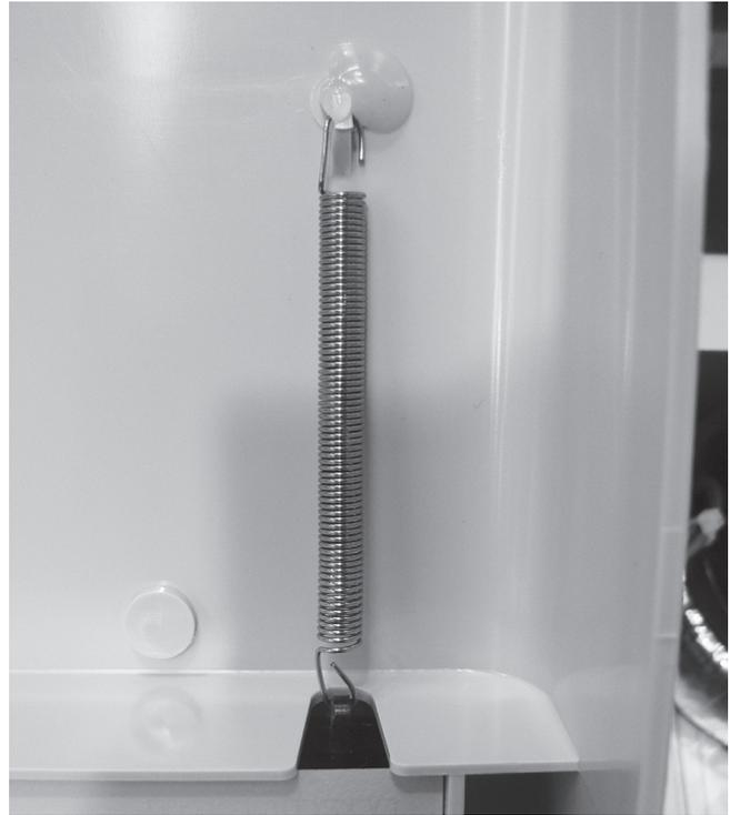
**Step 2** – Reattach spring to clip located on inside of chlorinator.
