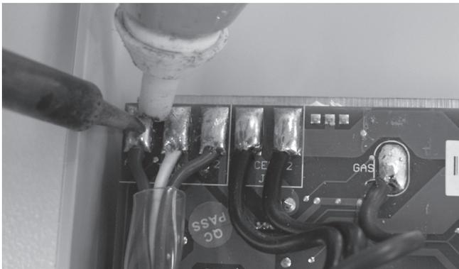
**Step 3** – With a soldering iron & solder sucker or solder wick remove all the wires for the cell cables, gas sensor & transformer.
