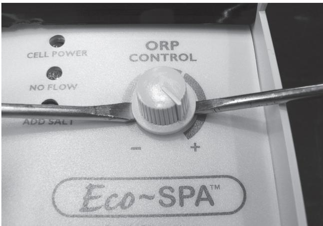
**Step 3** – Remove the ORP control knob which will allow you to move the PCB to the side. May need to use two flat blade screwdrivers to lever the knob off if it is fastened too tight to remove by hand. If using screwdrivers be careful not to damage the control panel.
