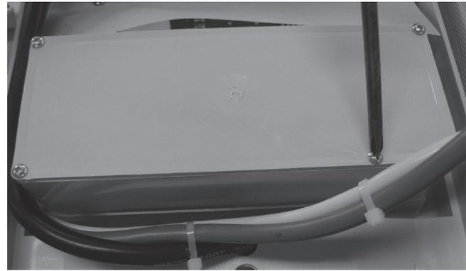
**Step 4** – Replace the covering on the terminal box using a Phillips head screwdriver (one point).
