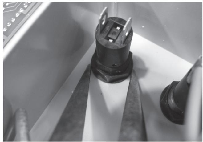
**Step 2** – Replace the nut that holds the fuse housing in place & tighten using long nose pliers.
