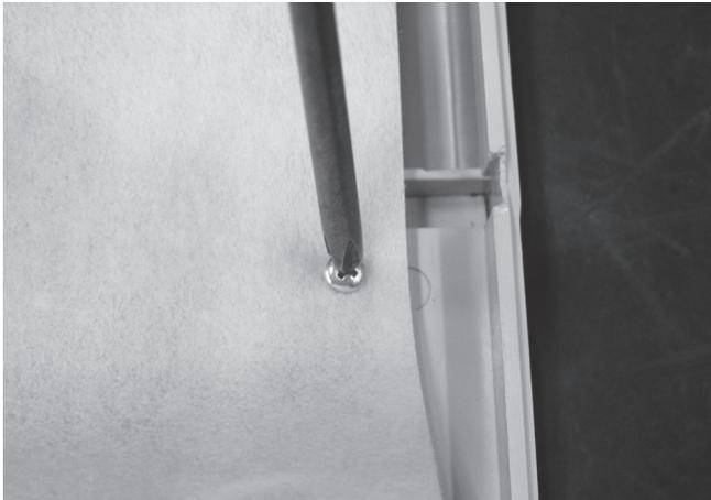
**Step 1** – Remove the screws holding the protective cover on the PCB with a Phillips head screwdriver (one point).
