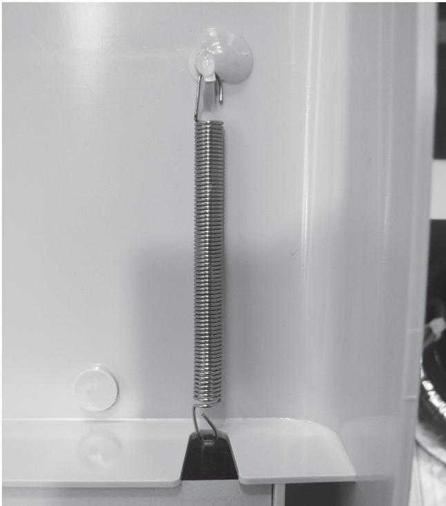
**Step 3** – Manoeuvre the spring so that it is able to be unhooked, may need to use long nose pliers to enable this.
