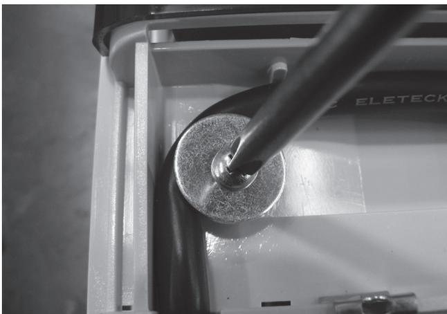
**Step 2** – Place cell cord assembly into position & secure with the holding plate using a Phillips head screwdriver (two point).
