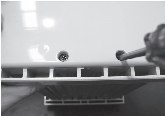
**Step 1** – Replace the screws holding down the top panel using a Phillips head screwdriver (two point) & press tabs back into place, (Part number M1500GRY).
