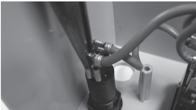
**BMSC 16/20/26 110V:** The lower terminal on the fuse has the brown wire from the bottom right slot on the terminal strip connected to it & the brown cable on the top terminal comes from the top left terminal on the power switch.
