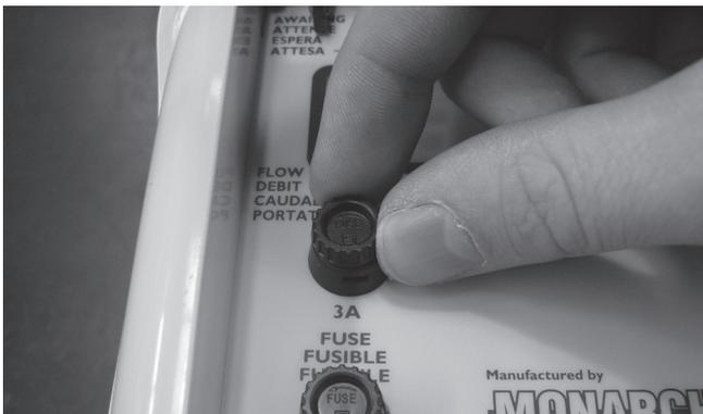
**Step 1** – Push down on the fuse & twist to the left.
