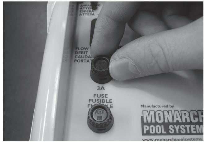
**Step 4** – Remove the fuse housing.
