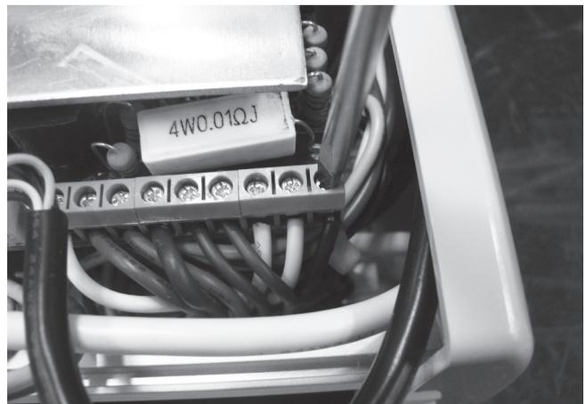
**Step 4** – Remove the wires connecting the transformer to the PCB using a flat blade screwdriver (3mm).
