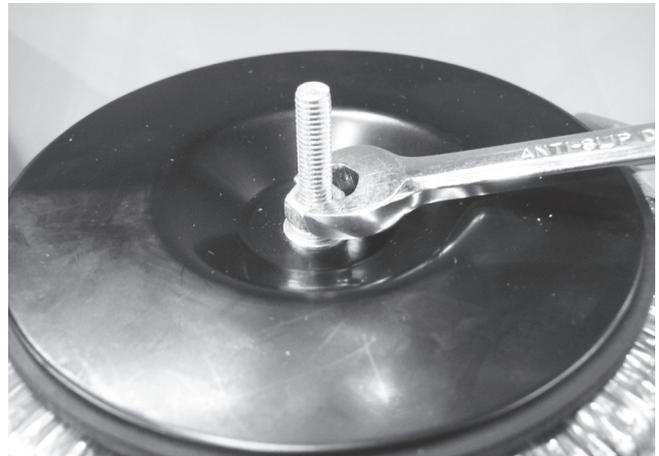
**Step 2** – Place heat dispersion disk over the transformer with the shiny metallic side face up. Place flat washer & spring washer in place over the locating screw; tighten the transformer nut using an 8mm spanner.
