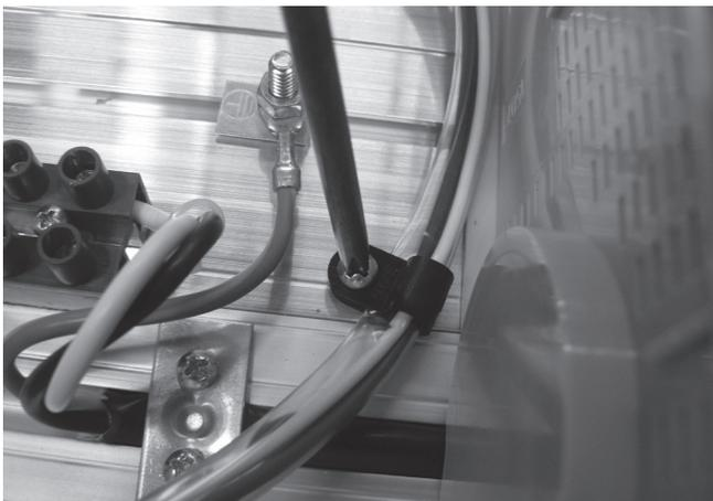
**Step 3** – Remove wire clamp holding the transformers secondary wires in place on the chlorinator using a Phillips head screwdriver (two point).
