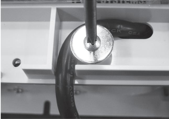
**Step 1** – After opening the front panel of the chlorinator use a Phillips head screwdriver (two point) to remove the holding plate allowing the cell cord assembly to be more easily manoeuvred.
