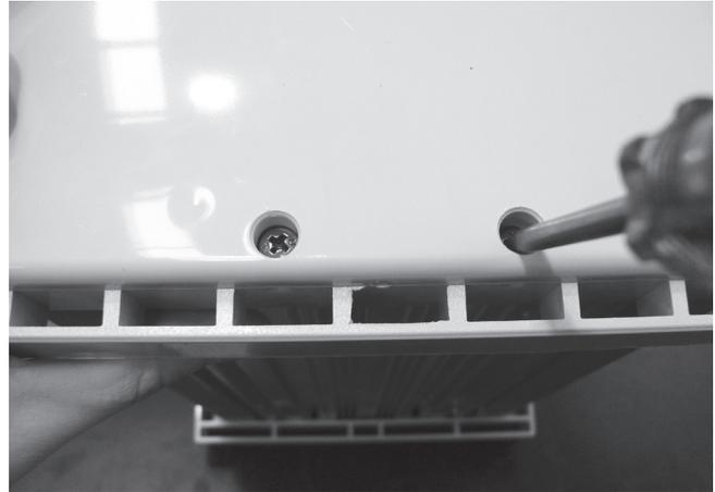
**Step 2** – Remove the screws holding down the top panel using a Phillips head screwdriver (two point).
