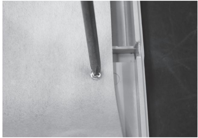
**Step 4** – Replace the protective covering on the PCB using a Phillips head screwdriver (one point).
