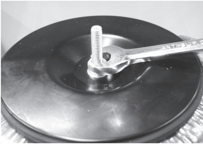
**Step 5** – Remove the nut on the top of the transformer with an 8mm spanner then lift off the black heat dispersion disk which when removed allows for the transformer to be lifted out of the chlorinator. When removing heat dispersion disk also remove the spring washer & flat washer located beneath the nut.
