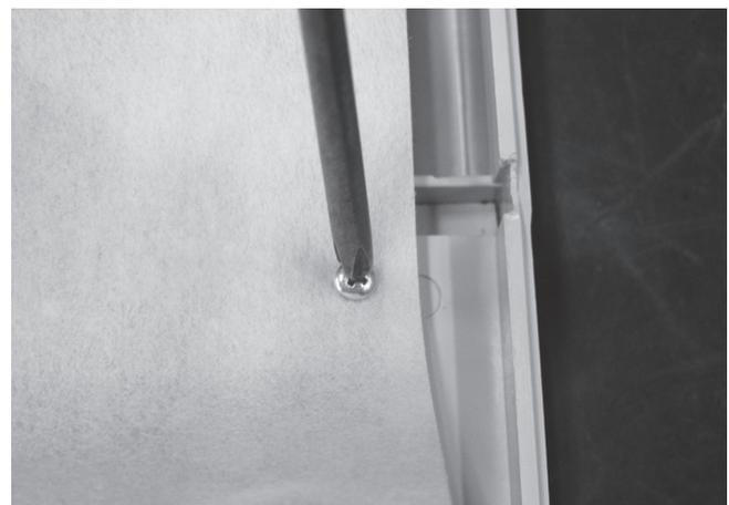
**Step 5** – Replace the protective covering on the PCB using a Phillips head screwdriver (one point).
