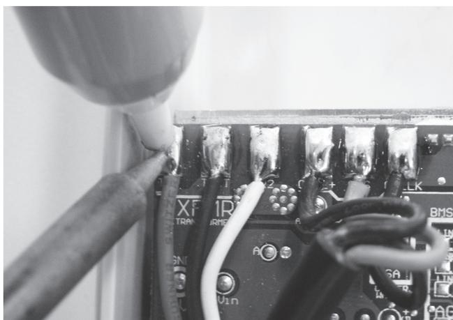
**Step 3** – With a soldering iron & solder sucker or solder wick remove all the cables connected to the PCB.
