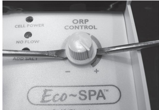
**Step 2** – Remove the ORP control knob which will allow you to move the PCB to the side. May need to use two flat blade screwdrivers to lever the knob off if it is fastened too tight to remove by hand. If using screwdrivers be careful not to damage the control panel.
