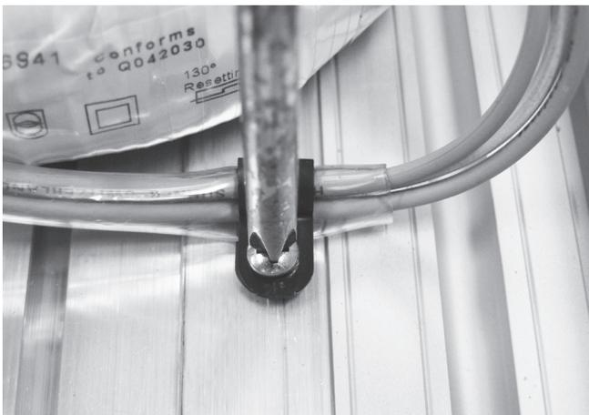
**Step 3** – Remove the cable clamp holding down transformer cables using a Phillips head screwdriver (two point).
