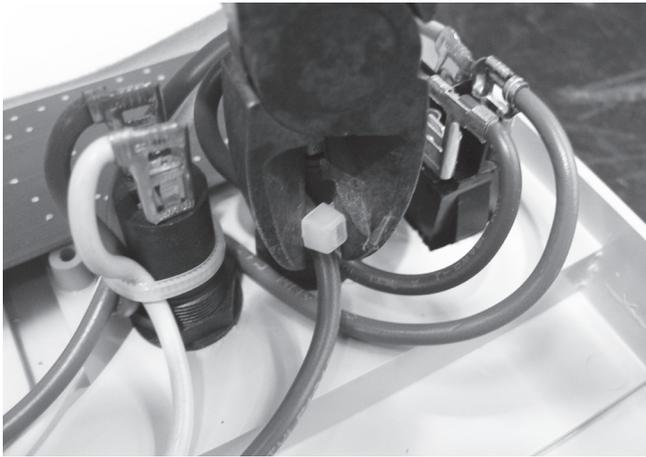
**Step 1** – Remove the cable ties holding the fuse wires in place with a pair of side cutters. Take special care not to cut or damage the wiring.
