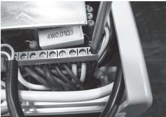
**Step 3** – Remove the wires connecting the various components of the chlorinator to the PCB using a flat blade screwdriver (3mm). Mark the wires to enable easier connection on reassembly.
