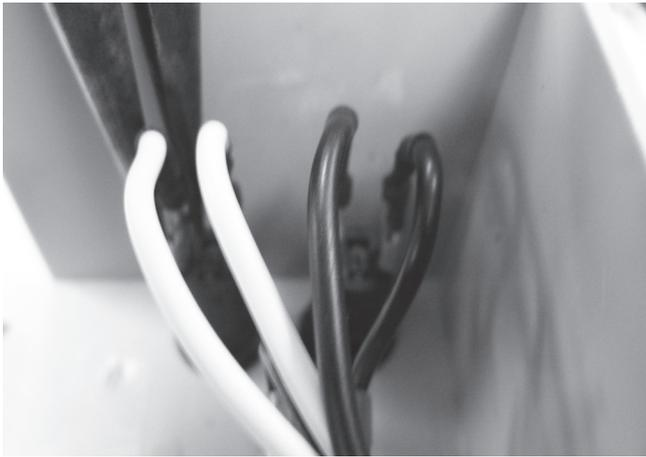
**Step 1** – Using long nose pliers remove all the clips from the fuse housing terminals. Mark the positioning of the wires to assist with reassembly.
