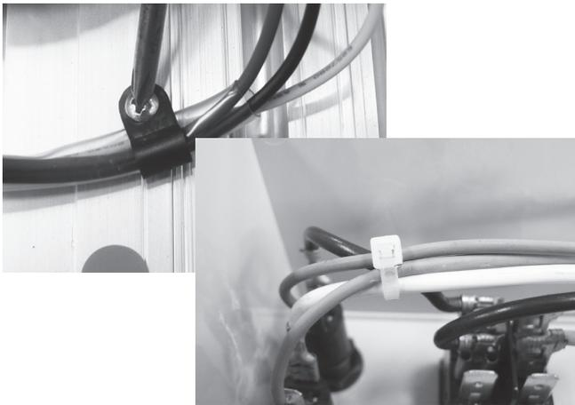
**Step 5** – Tighten cable clamp using a Phillips head screwdriver (two point) & replace any cable ties that were removed.
